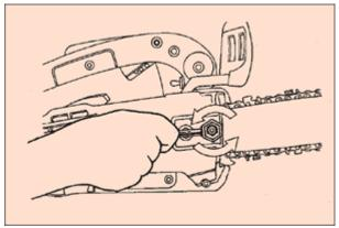
Fig 26: Loosening the bar-mounting nuts
