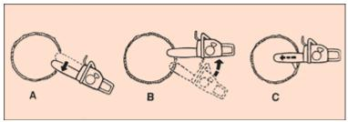
Fig 23: The boring cut - for experienced operators only.
