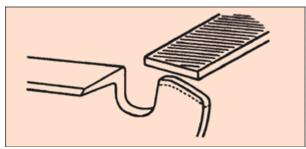
Fig 40: Maintain original shape of the depth gauge.
