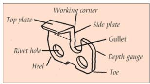
Fig 33: The parts of a cutter.
