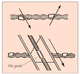
Fig 37: Use the file guide to maintain correct angle.
