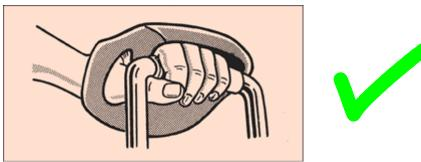
Fig 5: Chainsaw mitt helps keep your hand on the handle.
