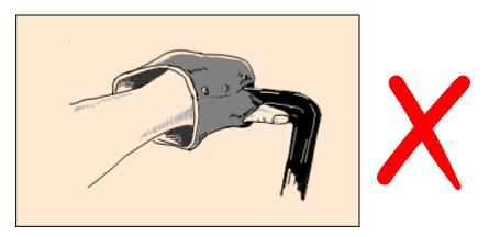
Fig 6: Thumb in an extended and potentially unsafe position
