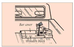
Fig 2: Secure chainsaw safely for transportation.
